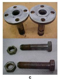
FIGURE 3 – SaltSpray/SO2 Gas Testing Results: a) Flange assembly before exposure, b) Flange Assembly Parts – Control – No FPS Protection, c): Flange Assembly Parts – Test – Two-Layer FPS Protection
