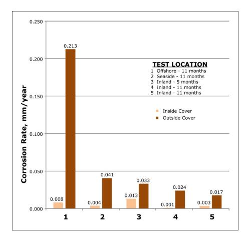
FIGURE 4 – Corrosion Rates of Metal Specimens – Brazil Locations
