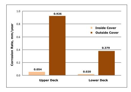
FIGURE 5 – Corrosion Rates of Metal Specimens – Singapore Location
